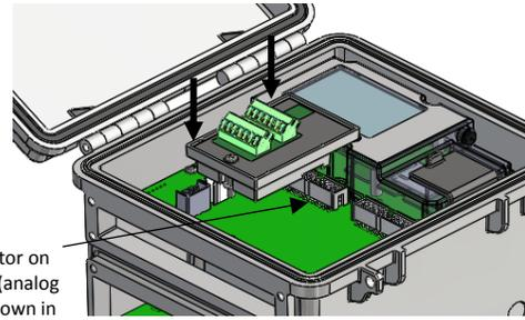
Insert the connector on the module here (analog sensor module shown in this example)
