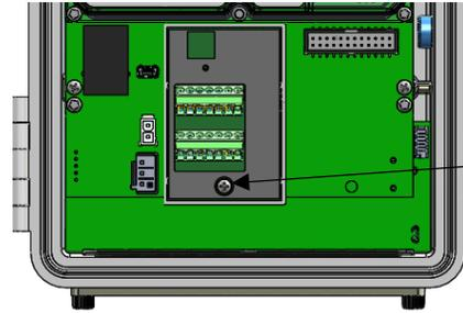
Tighten the screw on installed module
