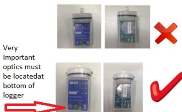
Very important optics must be located at bottom of logger
