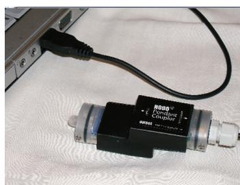
Make sure that the logger is inserted in the end of the coupler that has the magnet, and that the ridges on the base station and logger are aligned with the grooves in the coupler. If the logger is not aligned with the magnet, or if the ridges on the logger and base station are not aligned with the grooves in the coupler, the logger and the Optic USB Base Station will be unable to communicate.
