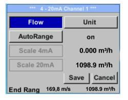
The 4-20 mA Analogue output of the Sensor VA 521 can be individually adjusted.
