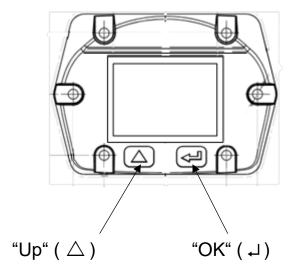
The operation of the VA 521 is done by the two capacitive key buttons Up  $(\triangle)$  and Enter  $(\ldot)$
