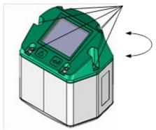
The Position of the Display head is twistable by 180 e.g. in case of reverse flow direction.
