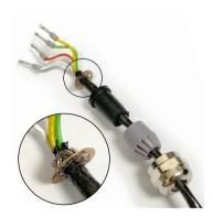
Ensure the cable shield braid is folded back over the cable jacket and gripped by the metal shield ring. This ensures a good electrical connection to the cable gland. 2. Thread the wires through the gland and re-connect them to the screw terminals.
