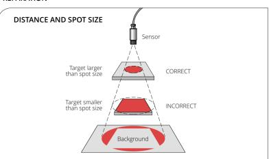
Ensure that the sensor is positioned so that it is focused on the target only. The size of the area (spot size) to be measured determines the distance between the sensor and the target. The spot size must not be larger than the target. The sensor should be mounted so that the measured spot size is smaller than the target.
