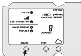
Press the Select button on the station to switch to the module with the manager (module 2 on RX2105 or RX2106 stations)
