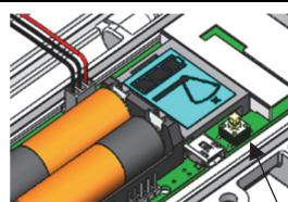
Open the sensor node door and install the rechargeable batteries. Press this button on the sensor node for 3 seconds.
