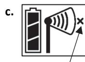
This network connection "x" icon blinks while the sensor node completes the registration process, which may take up to five minutes.
