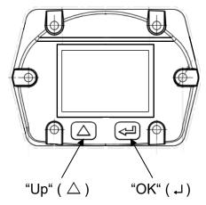
The operation of the FA 500 is done by the two capacitive key buttons Up ( $\triangle$ ) and Enter ( $\downarrow$ )
