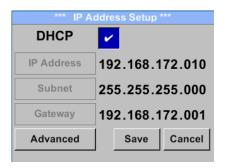
Here you can set up and made a connection, with or without *DHCP*, to a computer.
