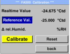
Here, a one-point calibration can be performed
