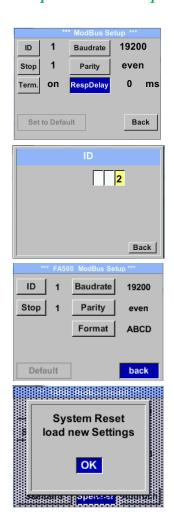
For changes, e.g. the sensor ID, first select by pressing key  $\triangle$  the field "ID" and then key "OK".
