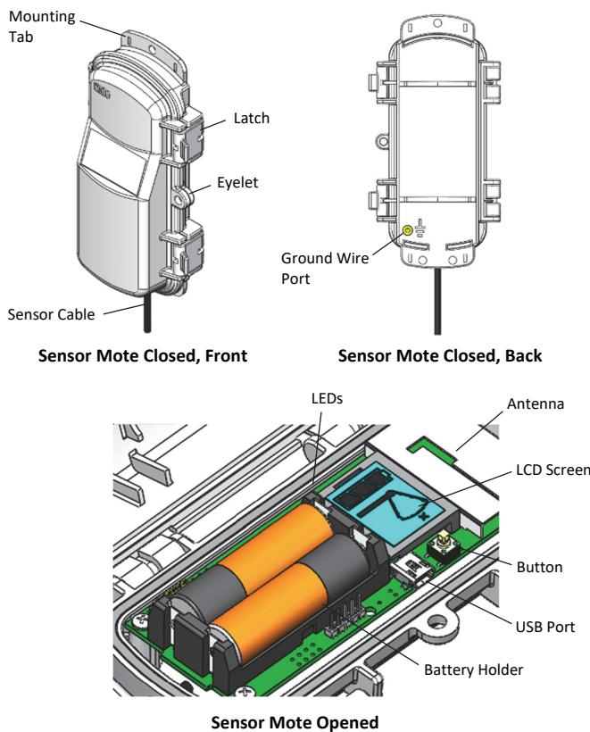
**Mounting Tab:** Use the tabs at the top and bottom of the mote to mount it (see *Deploying and Mounting*).
