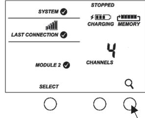
Press this button so the station is ready to have motes join the network
