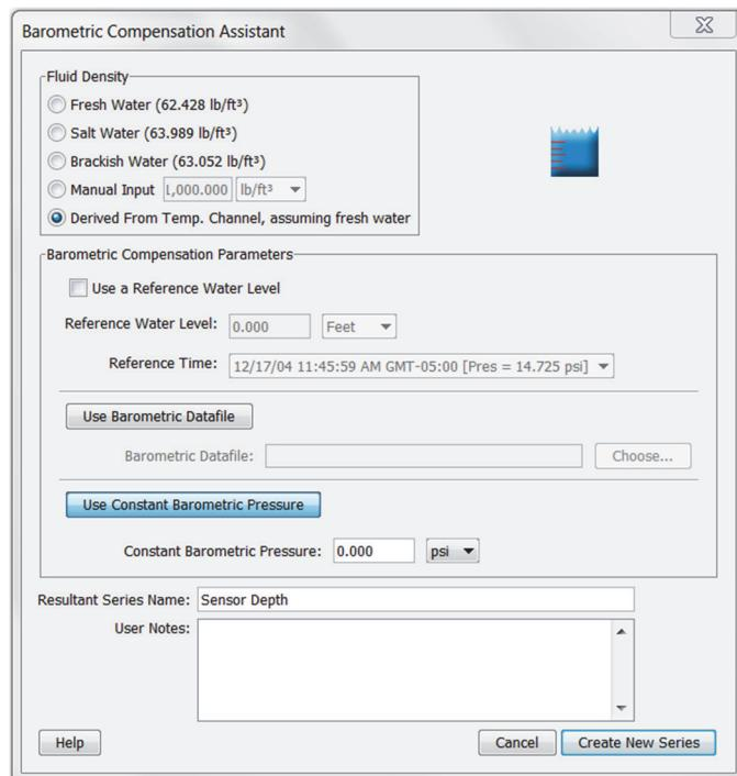
4. To enter a reference water level, check the Use a Reference Water Level box, enter the water level, and indicate whether it is in feet or meters.
