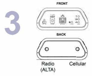
Connect the antennas to the back of the gateway as seen in the diagram.
