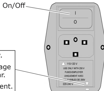
Check the fuse is installed correctly.
