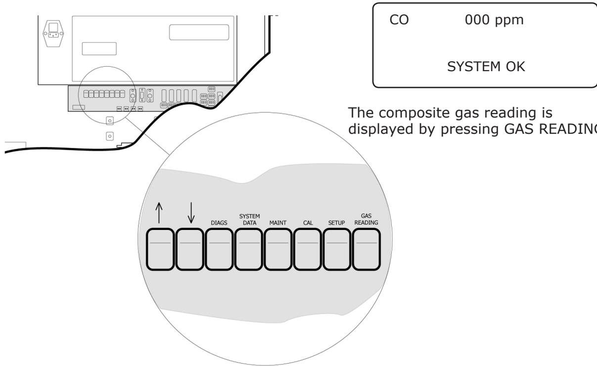
The composite gas reading is displayed by pressing GAS READING.
