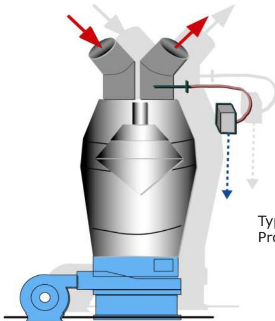
Typical installation of Mill Probe in a Classifier Outlet
