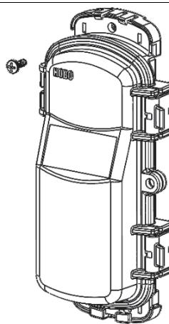
Close the sensor node and use a padlock to keep it secure.
