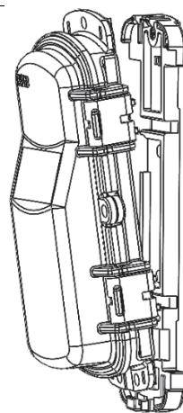
Use the short screw included in the package to fasten the sensor node to the bracket.
