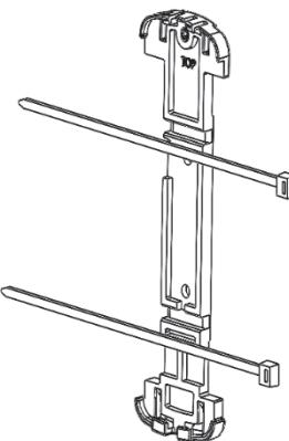
Insert the bottom of the sensor node into the retaining clips on the bottom of the bracket then press the top of the sensor node into the clips at the top of the bracket.
