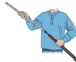
4. Use a repetitive up-then-down motion on the slide hammer to vertically drive the pilot rod into the soil.
