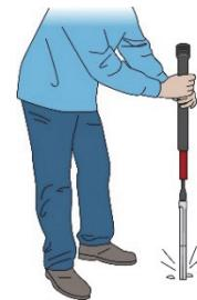
5. Once the pilot rod reaches the desired depth, extract the pilot rod by using the slide hammer in reverse, lifting it rapidly to hammer upwards.
