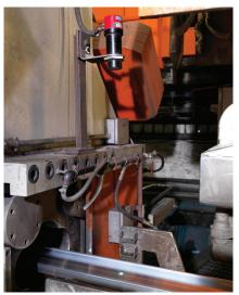
on the pyrometer or remotely using the integrated webserver via TCP/ IP with a standard web browser, the pyrometer measures an accurate product temperature for approximately 90% of all aluminium alloys, without the need for additional adjustments.
