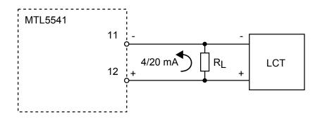
Configuration B:  $180 \Omega \le R_L \le 580 \Omega$  (using the internal resistance)
