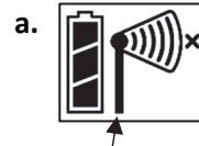
This signal strength icon blinks while searching for a network.
